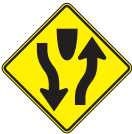
Start of Divided Highway
