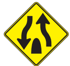
End of Divided Highway
